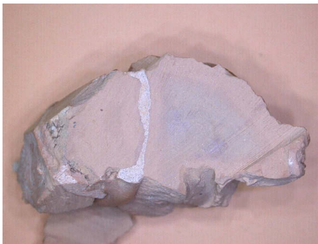
Fig. 1. The cross-section of the geopolymer joint between two ceramic–terracotta bodies.
